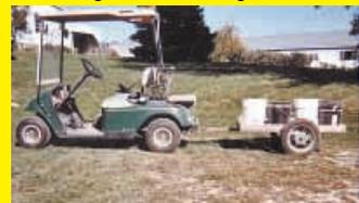
saves a lot of wear and tear on our tractor. The trailer rides on a pair of 16-in. motorcycle wheels, with a long threaded shaft serving as the axle. The bed is made from 2 by 4's mounted on an angle iron frame, the floor from expanded metal, and the tongue from lightweight sq. tubing.
