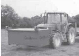
Portable workbench mounts on a front or rear 3-pt. hitch and can hold a welder, pto generator, and many other tools.
