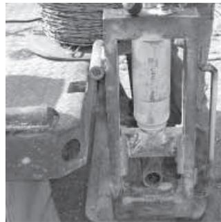
Electric/hydraulic portable pipe flattener was built from a used cylinder and scrap steel.
