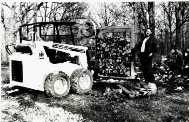
Wood is stacked in baler frame, pressed together hydraulically, then wrapped with steel tape.
