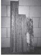
I drill a screw into the top of the board and place a spring on it, and also drill a screw into the bottom. Then I wrap one end of the chain around the bottom screw and connect the other end to the spring. Tension from the spring keeps the chain tight at all times. It's a quick and easy way to keep chains straight so they stay clean and are always ready to go."
