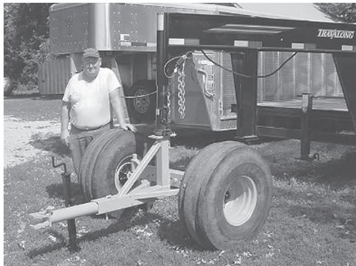
Schweppe took the wheels and axle from the back of a 750 Massey Harris combine and mounted them closer together. Then made a drawbar to pull it.
