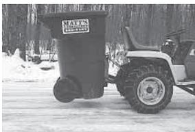
Angle iron, attached to top link, fits over handle on back of garbage bin.
