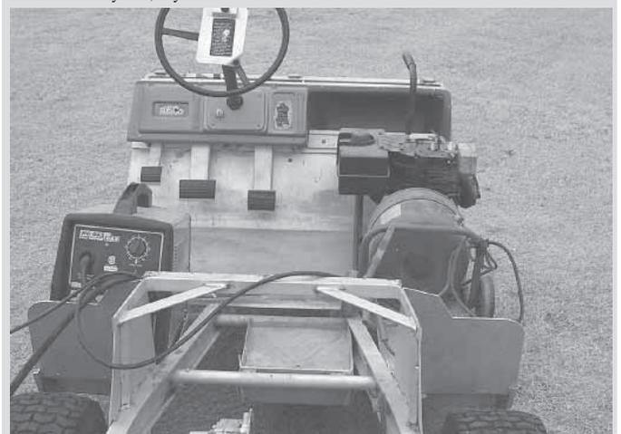
Patent-pending machine is designed to make mobile repairs and to provide emergency lighting and communications.
