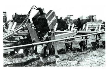
Individual Dewpoint subsoilers can be mounted on chisel or moldboard plows to combine two operations into one.
