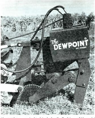
About 16 hp are required to drive hydraulically-driven orbiting point of the Dewpoint subsoiler, which operates 12 in. underground. Unit can be mounted on a 3 pt. hitch, or several units can be ganged on a toolbar.
