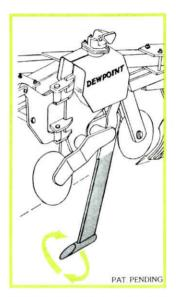
Subsoiler's bullet-shaped point is angled 30° and orbits at 1400 rpm's to "fracture" compacted soil in path 8 to 10 ft. wide at a depth of 24 in.
