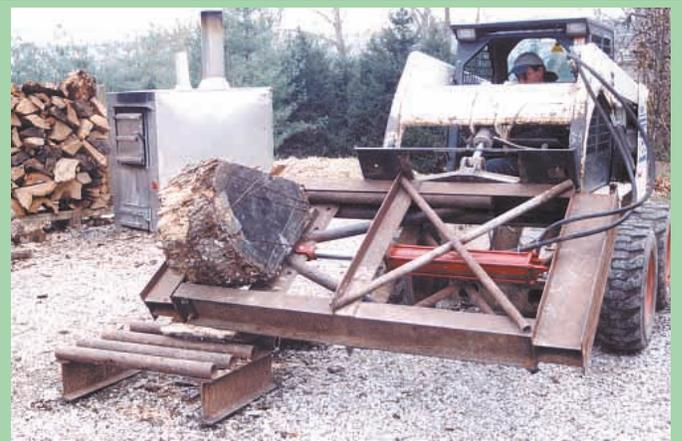
Splitter is built from 8-in. lengths of bolted-together I-beam. It measures 6 ft. long and 3 1/2 ft. wide.
