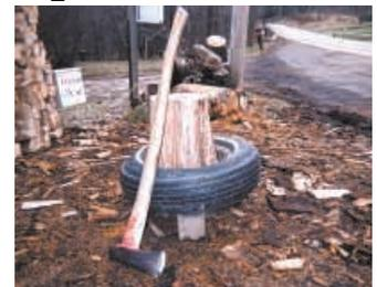
Karg drives two stakes into the ground and then makes slits in the bottom sidewall on a tire to slip over the stakes. The stakes push against the top sidewall which is not slit.
