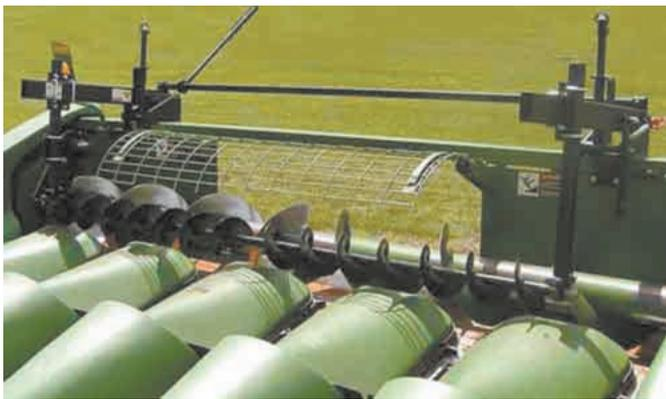
Auger attaches to Deere 90 series corn head frame using clamp-type fasteners. The system is self-contained and operates off a hydraulic motor.
