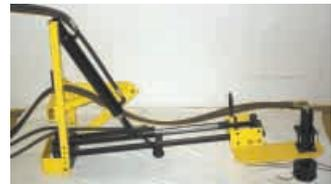
It's powered by tractor hydraulics and will trim a 24-in. dia. circle.
