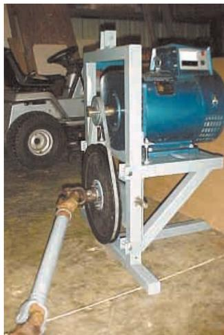
Madison found a generator on eBay and made a frame to pto-power it on a 3-pt. hitch.
