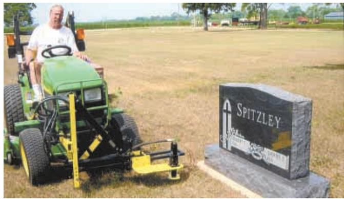
Spitzley used scrap parts to build the string trimmer. "From the seat of the tractor, the head can be adjusted 1 ft. in any direction," he says.
