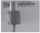
Solenoid-activated valve plumbs into gas line and wires into the ignition switch to automatically shut off the gas valve when the ignition shuts off. With a few modifications, it'll work on most antique tractors.
