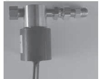
Solenoid-activated valve plumbs into gas line and wires into the ignition switch to automatically shut off the gas valve when the ignition shuts off. With a few modifications, it'll work on most antique tractors.
