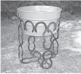
Plant stand (above left) is 2 ft. in dia. and 3 ft. high. It's made from 36 horseshoes. The "welcome" in the sign (above right) was formed by welding 9 horseshoes onto an old scythe blade.
