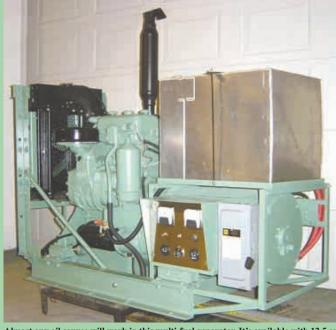
Almost any oil source will work in this multi-fuel generator. It's available with 12.5 or 20 KW output, which will provide plenty of power for most homes, small businesses, and farms.
