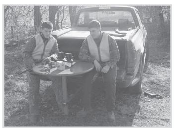
The "TableGater" is a 36-in. dia. wood table that fits on a length of sq. tubing that slides into pickup receiver hitch.
