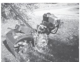
Colin Plasch uses an old rototiller to power a pressure washing pump, which fit the bolt pattern and driveshaft on the tiller.
