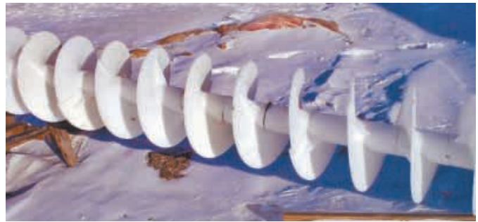
The Compo*Starr system uses a 20-in. auger inside a 24-in. plastic tube to mix manure and ground-up corn stalks.
