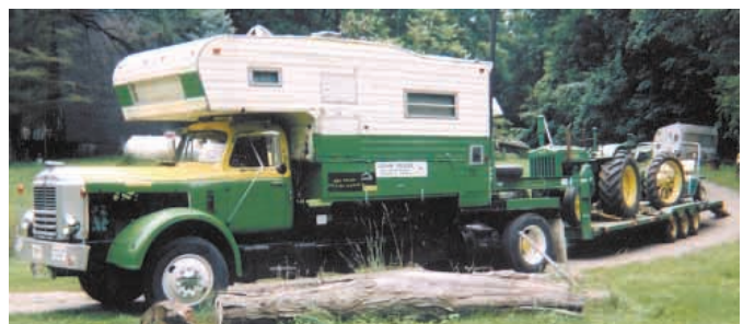
Hank Friday converted a 1967 Hendrickson semi tractor into this motorhome by mounting a 10 1/2-ft. long pickup camper on back. He pulls a 35-ft. long trailer behind it.
