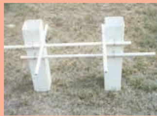
Simple box inserts fit neatly into the square holes in bottom of drill box. Each insert holds about 12 lbs. of seed.
