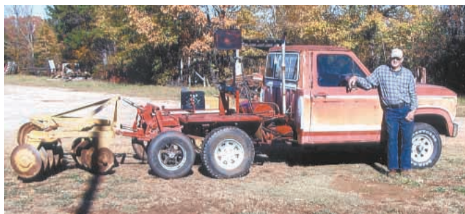
W.T. Elliott modified this Ford F-150 by mounting a 3-pt. hitch and dolly wheels on back. Lets him haul bales down the road at 50 mph, or even do light disking.
