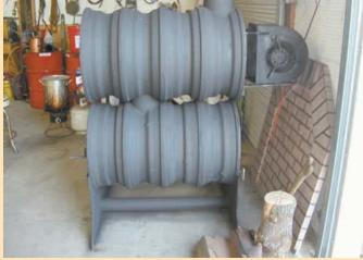
Gary Tickner built this stove by cutting the centers out of four 25-in. truck wheels and welding the rims together for a firebox. He cut flat plates for both ends and made a door in one end. He cut four air inlet holes in the door and in the rear plate, mounting sliding plates with offset holes over both to act as dampers.
