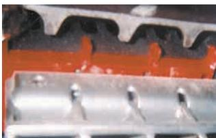
Add-on "stripper knife" is designed for the rotors on IH 40, 60, and 80 series combines.
