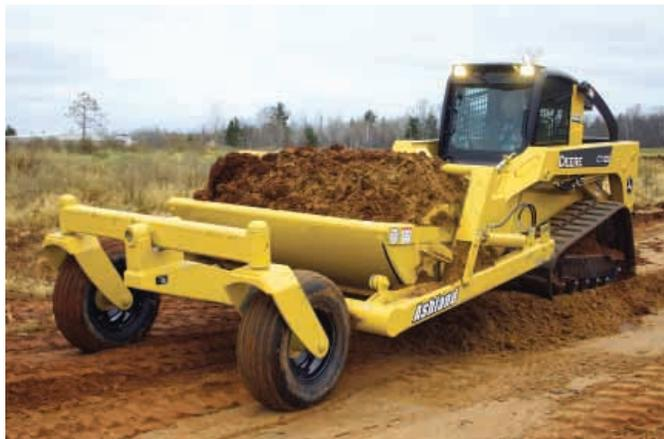
Ground Hog scraper mounts to the quick-tach plate on skid steer loader arms. Caster wheels on front end help carry three to four times the load a conventional bucket could handle.
