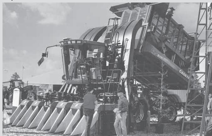
Case IH introduced its Module Express 625, which produces compressed square bales.
