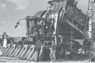
Case IH introduced its Module Express 625, which produces compressed square bales.
