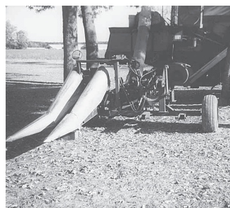
Johnny Mooring built this 3-pt. mounted, one-row snapper head out of a 5-row corn head and a grain table off a Gleaner M3.
