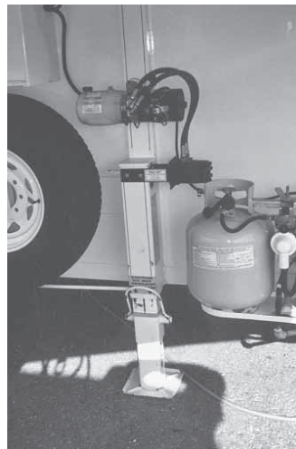
Hydraulic-powered attachment turns any hand-cranked trailer jack with ease, says J.L. Sharp.
