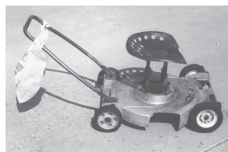
Metal tractor seat mounts on top of push-type mower with its blades and engine removed.
