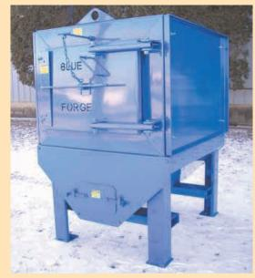
"Blue Forge" gasification stove got its name from the forge-type fire it creates, caused by an "upside down" burn. The unit smokes less because it burns the emissions coming down from the primary firebox in a secondary burn chamber, where air is injected. In the primary firebox (right), wood goes through an intense baking process that pulls out the gases and burns them as they're forced down through a coal bed.
