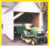
Using my Deere X485 garden tractor and a home-built dump trailer, I was able to move an 8 by 12-ft. storage shed about 100 ft. to a concrete slab next to my shop. To move the shed, first I bolted three planks on the vertical studs. Then I jacked the shed up 5 in. and backed the trailer under it and used welding clamps to clamp the planks to the top of the trailer. Then I pulled the shed to the spot and set it down.
