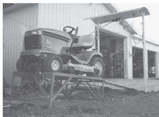
Deck washing system uses a pivoting spray arm to which a garden hose is attached.
