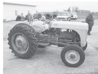
Kit costs \$995 and contains all the hardware needed to connect the V-8 engine and clutch assembly to the Ford 8N transmission and frame. Knasel says it takes about 8 to 10 hours to install.
