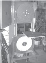
Using a lathe and milling machine, Bruce Chandler built his own metal-cutting bandsaw.
