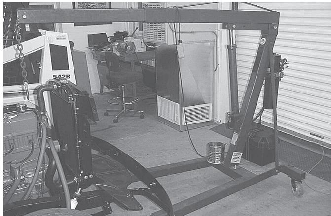
**Sladky modified this engine hoist to respond with finger touch control.**
