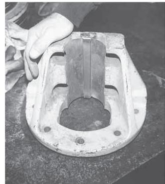
**To restore worn wheel hubs to "like new" condition, Dale Denton cuts a new keyway into the wornout hub and replaces it with a new full-size key.**
