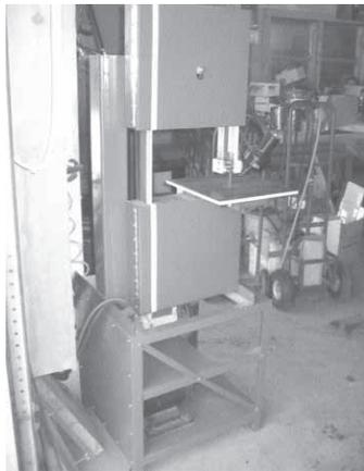
**Using a lathe and milling machine, Bruce Chandler built his own metal-cutting bandsaw.**
