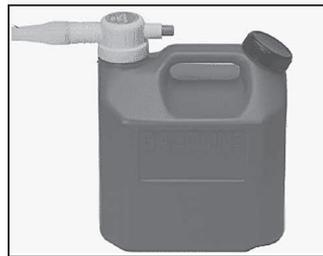
to 3 gpm. The self-venting nozzle stops the flow of fuel when the target tank reaches full. The can has a single opening for filling and pouring. Available in 1 1/4, 2 1/2, and 5-gal. size cans. A variety of spout extensions are available.
