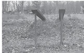
key' ramps. They work great for changing oil on vehicles, removing the blades from my riding mower, and many other jobs. The ramps are set up on a slight hillside, with one end of each I-beam lying on a pile of dirt. The other ends are supported by a steel post
