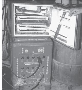
to be just the right size for storage of welding rods. I keep it on top of my welding machine.
