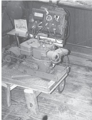
charging system. It works great for charging any vehicle with a dead battery. All the information on the wiring schematics that's required to build this charging system can be found in any auto repair manual.
