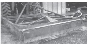
Hinged box blade on back extends about 2 in. below four angled blades on front. Box blade is raised and lowered by a hydraulic cylinder that mounts in middle of frame.
