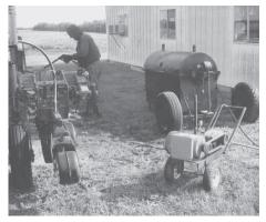
Homemade pressure washer mounts on a homemade, 2-wheeled cart. The pump is operated by a 5 hp electric motor.
