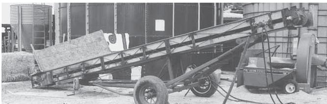
Elevator faces backward and its bottom "drive" end is raised just enough to unload silage into silo blower.
