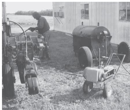
Homemade pressure washer mounts on a homemade, 2-wheeled cart. The pump is operated by a 5 hp electric motor.
