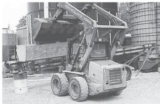
Baumann uses his skid loader to load silage from a sausage-type storage bag into the elevator to fill up the silo.
