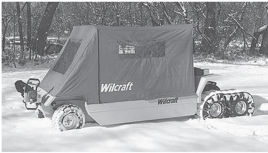
Wilcraft ice house is an amphibious vehicle that lets you drive to where the fish are biting. By pressing a switch you can quickly raise or lower the wheels.
