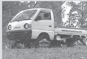
A mini truck fitted with tracks is offered by American Mini Trucks.
