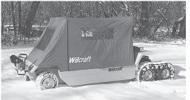
Wilcraft ice house is an amphibious vehicle that lets you drive to where the fish are biting. By pressing a switch you can quickly raise or lower the wheels.
