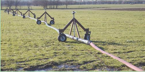
Towable system consists of nine caster-wheeled steel towers spaced about 40 ft. apart and equipped with nozzles on top. Tow carry a 4-in. dia., heavy duty poly pipe via metal braces clamped onto the pipe.
