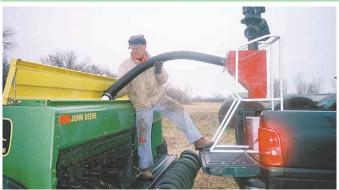
Powered by any commercial gas-fueled leaf blower, the Kwik Kleen double-chambered seed vacuum makes it easy to clean out seed boxes in drills and planters.
