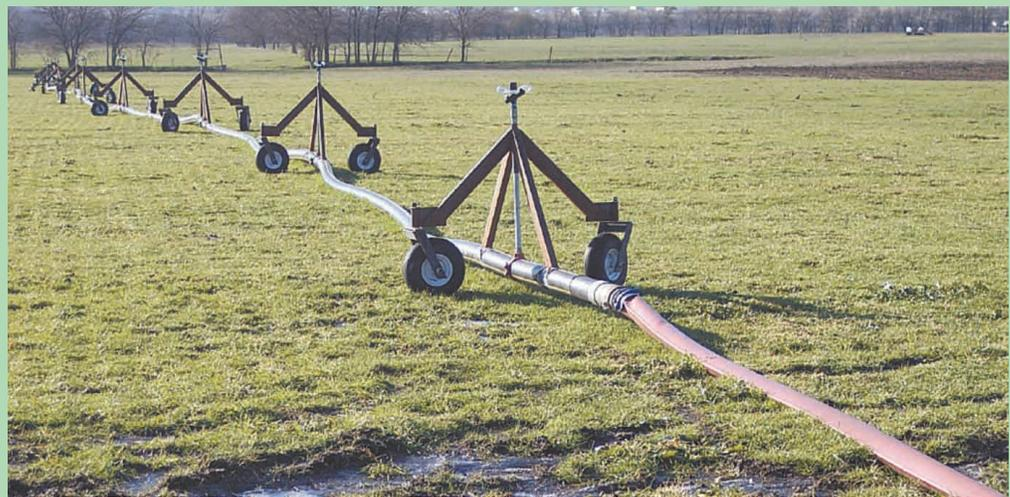
Towable system consists of nine caster-wheeled steel towers spaced about 40 ft. apart and equipped with nozzles on top. Towers carry a 4-in. dia., heavy duty poly pipe via metal braces clamped onto the pipe.
