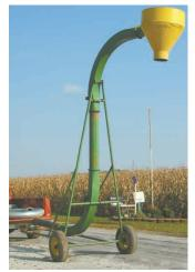
He replaced the flexible steel pipe that was originally attached to the cyclone with about 30 ft.of blower pipe. That increased the height of the cyclone by about 6 ft. for extra clearance when unloading grain into trucks and wagons.
