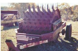
Massive aerator has a drum 5 ft. long and 5 ft. in diameter that's made of 1-in. thick steel.
