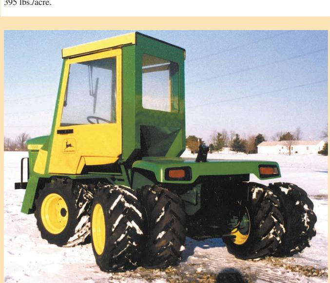
Front tractor is a Deere 318 model, and the back is a 317. Tractor’s eight wheels are off the original garden tractors.
