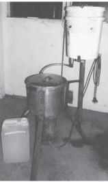
Bud Pitts built this centrifuge to clean waste vegetable oil to use in his converted Datsun diesel pickup.
