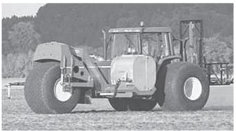
Front wheel kit turns any mid-size tractor into a 3-wheeled floatation sprayer.
