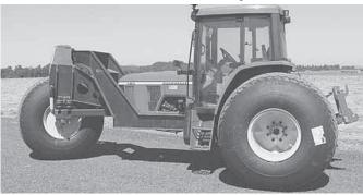
Tractor's rear wheels are replaced by 66-in. high, 44-in. wide floatation wheels.
