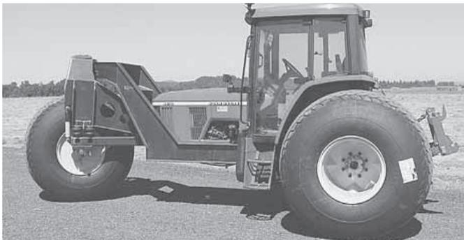
Tractor's rear wheels are replaced by 66-in. high, 44-in. wide floatation wheels.
