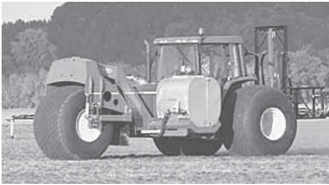
Front wheel kit turns any mid-size tractor into a 3-wheeled floatation sprayer.
