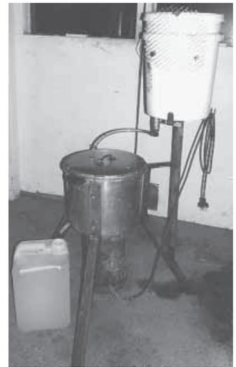
Bud Pitts built this centrifuge to clean waste vegetable oil to use in his converted Datsun diesel pickup.
