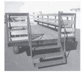
Wagon has three steel steps with hand rails on back. Bottom step is hinged and can be folded up out of the way.
