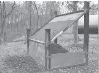
"It works great for removing rocks from topsoil that I scrape off my land," says Don Ickes about his home-built, portable topsoil screener.
