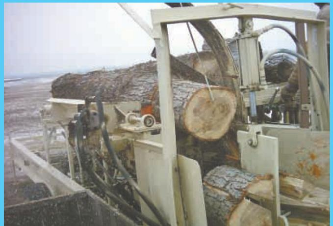
Log processor is powered by a Chevy 366 engine that came off a wrecked truck. It drives a hydraulic-powered chainsaw bar.
