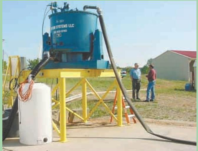
Centrifuge is designed to remove water before spreading manure. The automatic system requires no operator and can handle fresh flushed manure or older lagoon sludge.
