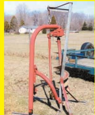
welded on top of the auger's mounting arm. Then I detach the auger from the tractor's 3-pt. hitch and lower the auger until it dangles above the ground. (Joseph L. Bellor, 2578 Reed Rd., Lapeer, Mich. 48446 ph 810 667-2854)
