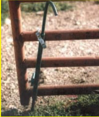
I made this simple gate holder that sticks in the ground to hold a gate open. It U-bolts to the gate when it's closed. I took a length of 1/2-in. square tubing and welded a 3/2-in. length of 1/2-in. rod to the top of it that I bent into a curve. I also welded a 5-in. piece of rod with a 90-degree curve at the bottom. It's a great time saver. (Walter E Bueker, 35570 Bueker Rd., California, Mo. 65018; ph 573 796-2558; wbueker@yahoo.com)
