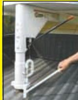
utes. You just drill two 1/4-in. dia. holes in the trailer gusset and adjust the length of a cable. Sells for \$39.95 plus S&H. It can be ordered at www.eze-latch.com or you can call toll-free 866 231-8589. (Arden Vernon, POB 356, Turon, Kansas 67583 ph 620 497-6475; www.eze-latch.com)
