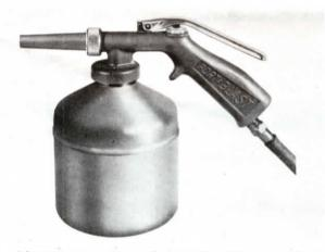
For larger jobs, one-qt. container can be set aside and the gun used with a siphon tube which draws abrasive material from a large hopper or bucket.
