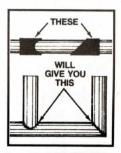
Patterns in the Welder's Helper kit are used to make saddle and elbow templates for any size pipe ranging from 1½ to 8 in. in dia.
