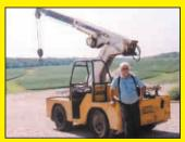
I found this 1954 self-propelled Case crane in the weeds and bought it for not too much. The engine was shot so I replaced it with a Ford V-8 engine and transmission. It was a tight fit but ended up working great. The engine was a 302 Ford out of a 1978 pickup. It's been a very handy machine around our place useful for a lot of jobs. (Charles Klein, Columbia, III.)
