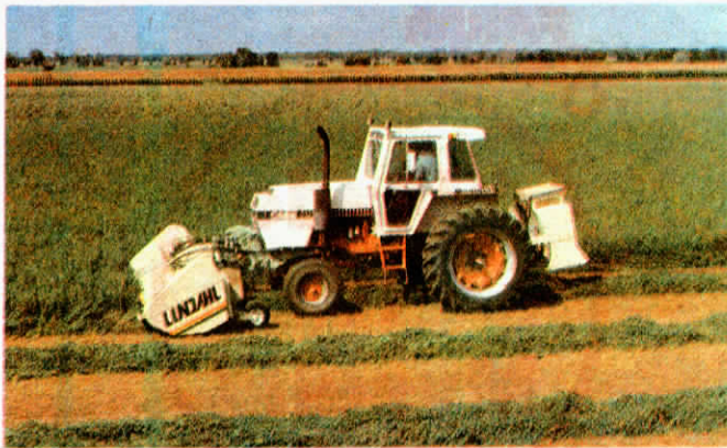
Rear-mounted hydraulic power pack lets you carry pto-powered 3-pt. equipment up front.
