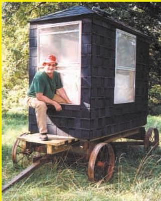
comfortable "executive" portable deer stand that he can roll around his acreage as needed. He lives in a densely wooded area by a highly traveled highway. There are a lot of deer. Using a steel-wheeled wagon gear, some salvaged plywood, and old aluminum windows, he made a heated stand with comfortable seating inside. He put the large windows on all four sides (he enters through one of them) and put a shingle roof on top. He puts curtains over the lower half of the windows so deer can't
