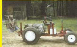
could find laying around my farm, including a 5 hp Briggs & Stratton engine and a 4-speed truck transmission from around 1940 with a chain drive to the axle. I built a combo gearbox chain drive for the steering.
