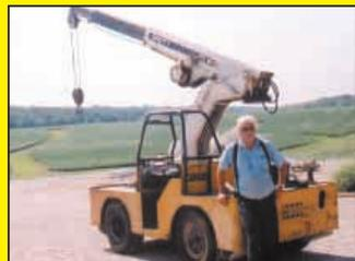
I found this 1954 self-propelled Case crane in the weeds and bought it for not too much. The engine was shot so I replaced it with a Ford V-8 engine and transmission. It was a tight fit but ended up working great. The engine was a 302 Ford out of a 1978 pickup. It's been a very handy machine around our place - useful for a lot of jobs. **(Charles Klein, Columbia, Ill.)**
