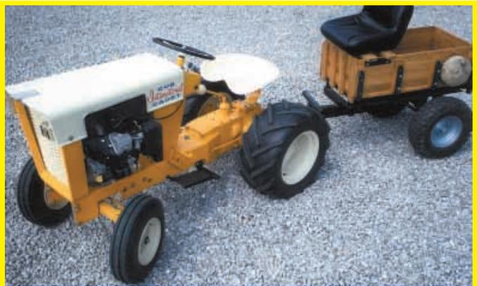
I was given a Cub Cadet 70 garden tractor if I would drag it out of a barn where it had been a target for pigeons. The 7 hp Kohler motor was stuck so I replaced it with an 11 1/2 hp Kawasaki pull-start. The original Cub generator/starter still worked so I mounted it on the main output shaft, removed the recoil, and machined a pulley to stick out 2 1/2 in. I had to drill only
