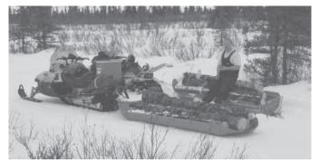
Sleds made from 1/4-in. UHMW poly come with triangular tongues for pulling behind snowmobiles, ATV's and other machines.
