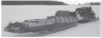
UHMW poly stays flexible at temperatures down to 60 degrees below zero.
